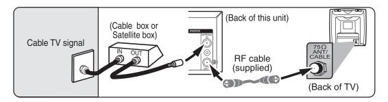
This connection allows you to view or record a scrambled channel. With this connection, channels cannot be changed on this unit. You can view or record ONLY the channels you have selected on the cable box or the satellite box. • While you are recording, only the recorded channel can be viewed.
